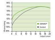
Emparro 3-phase has such a long life span because of its efficiency rating of up to 95%. The resulting power loss is very low which exposes the components to less thermal stress.
