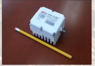
This smallest and lightest 2W L-To Ku-Band Block Up Converter is based on GaN technology and is designed to be mounted directly on the feed horn. High power efficiency resulting in low current (< 1 amps) consumption allows user to pass DC supply voltage via IF cable. The unit is ideal for network and point to point, data distribution, portable and emergency applications.
