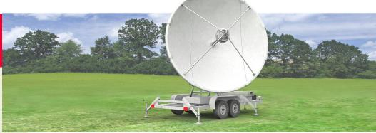
The antenna's Trifold® reflector panels are cut from a single-piece of precision spun aluminum.
